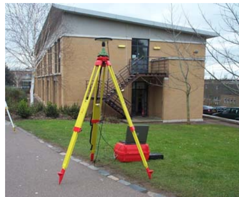
Figure 3: Test Location with Ublox L1 GPS Receiver and Thales Antenna
